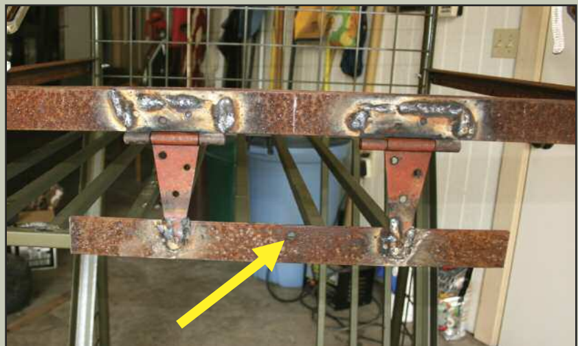
A ⅜-inch metal drill bit was used to drill this small hole into the trigger mechanism so that it can be attached to a trip wire.
