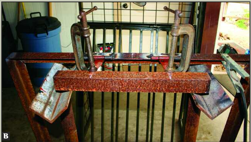
C-clamps secure two T-hinges to the bracket (A). Once secured, a welding machine is used to tack hinges into place. A small piece of angle iron is attached to the other side of the hinges to construct the trigger mechanism (B).
