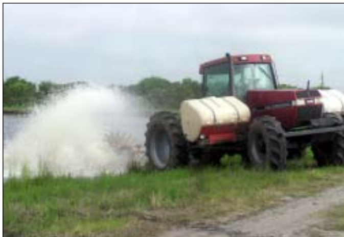
Figure 15. Tractor powered (PTO) "sidewinder" type paddlewheel aerator.
