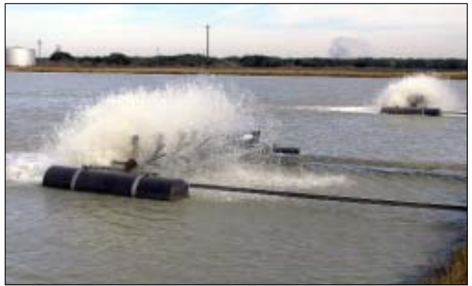
Figure 16. Electric paddlewheel aerators.
