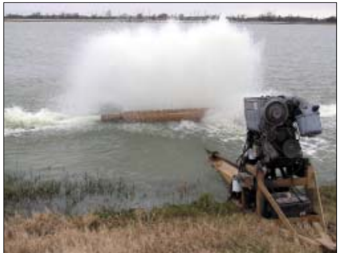
Figure 17. Pump-sprayer or "bankwasher" type diesel aerator.
