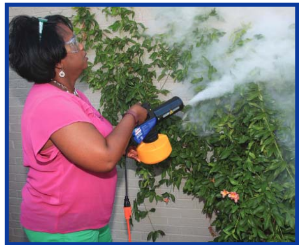
Figure 3. Small thermal fogger producing a dense fog to kill mosquitoes resting in backyard vegetation and shrubs. Fogs work best when applied in the evening or when there is little wind. Source: Mike Merchant
